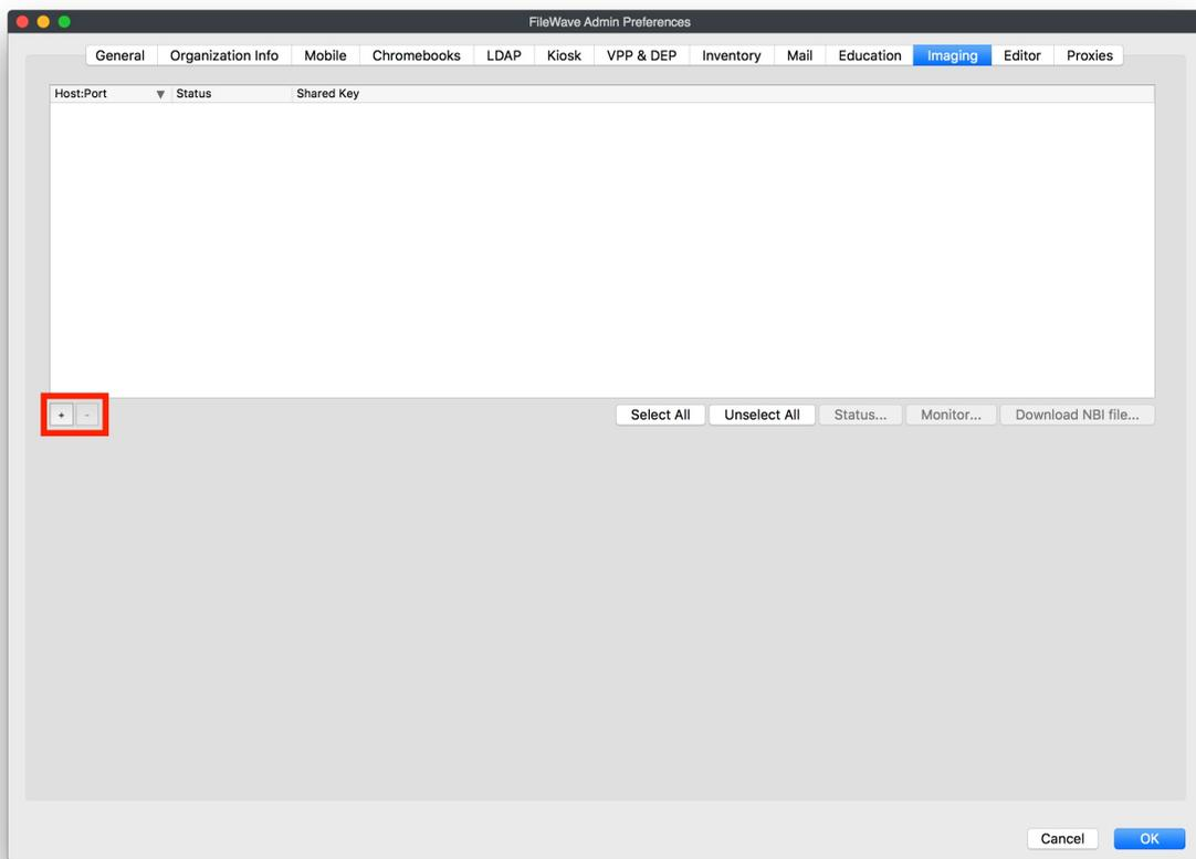
4. Enter the IP address of the IVS into "Preference for Imaging"
