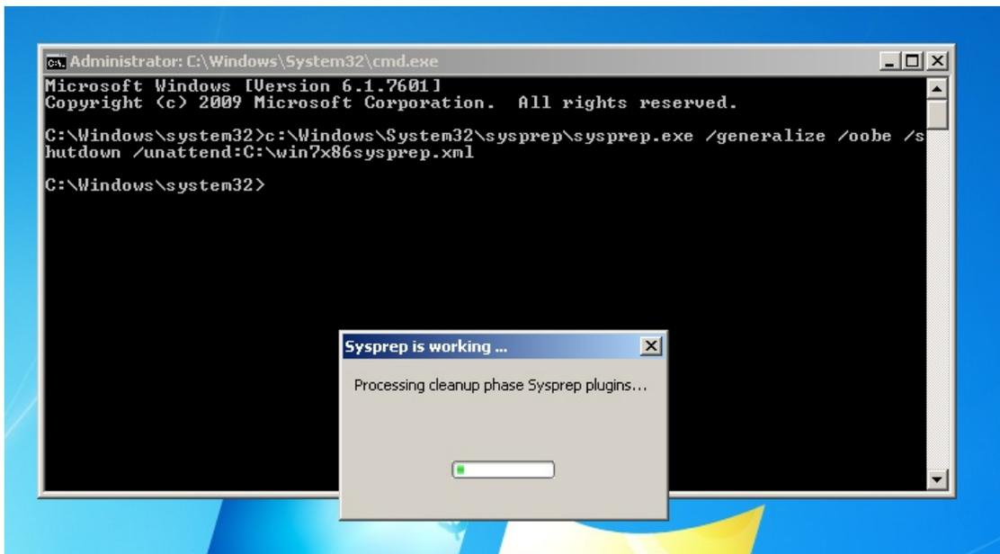
Sysprep will prepare the machine to be copied and shutdown. You are now ready to upload your Master Image to the FileWave Imaging Appliance.
